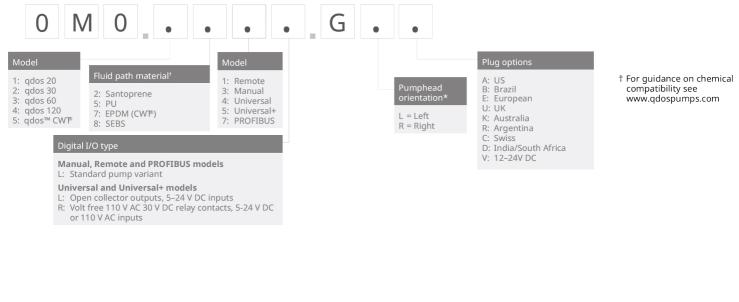
\* The pumphead side location is required when ordering. The left/right perspective assumes the user is looking at the front of the pump. The pump in the dimensions diagram is considered a pumphead located to the left.
